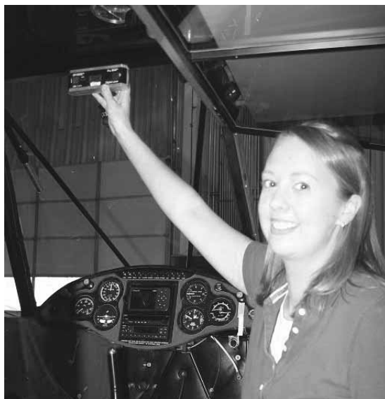
Figure 6-2 - Leveling the Aircraft
