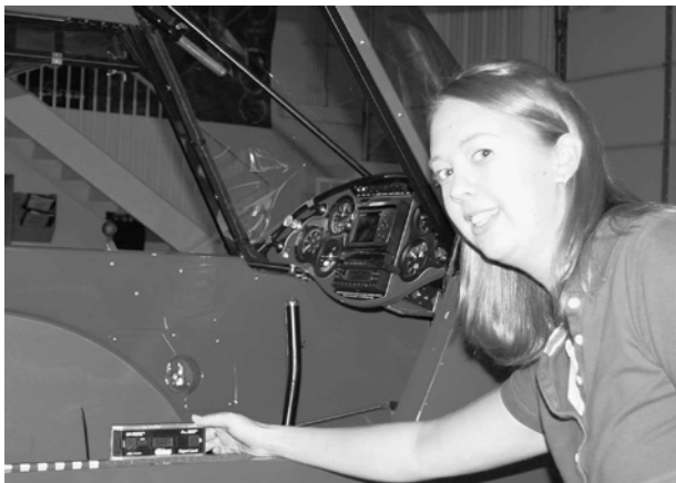
Figure 6-1 - Leveling the Aircraft
