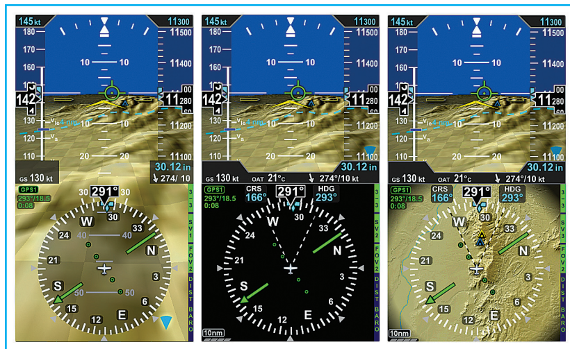
Figure 3-1 (left to right) PFD Full Screen (SV1), Split Screen with standard Nav Display (SV2), and Split Screen with Nav Display overlaying Topographical Map (SV3)
