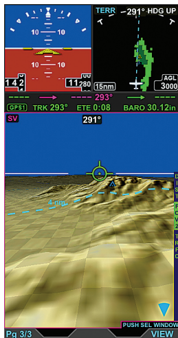
Figure 3-26 ESV in Bottom Window
