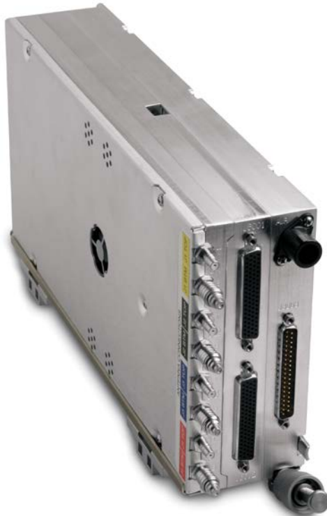
Figure 4 GTS System Processor
