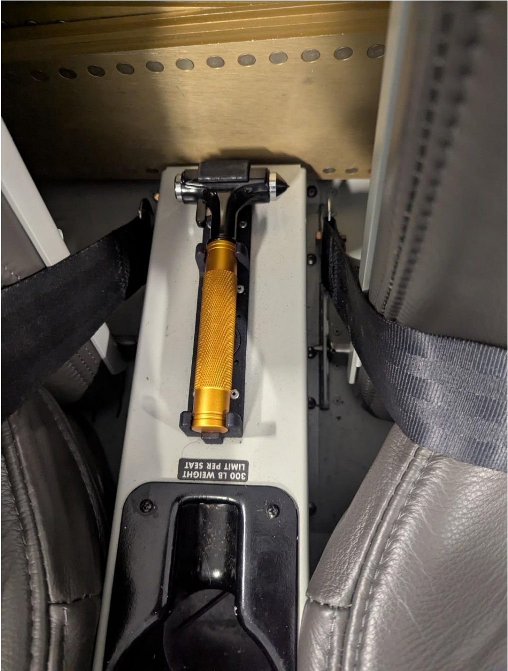
FIGURE 7-14 EXAMPLE EGRESS HAMMER LOCATION
