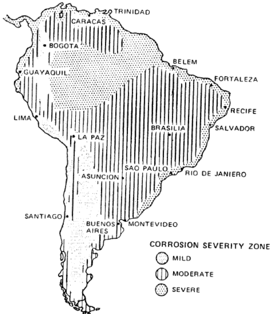
Figure 4-16: South America Corrosion Severity Map
