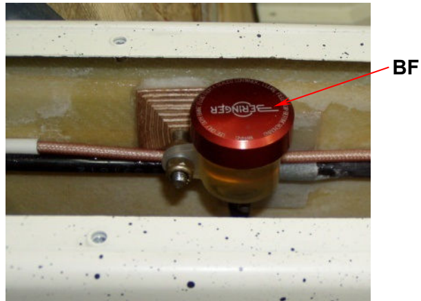
Fig. 2.2.8-2 Operating fluids - brake fluid
