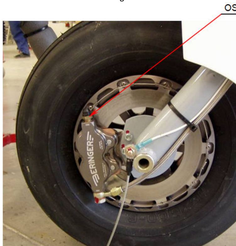
Fig. 2.2.4.2-1 Brakes venting (illustrative figure from model Speed)
