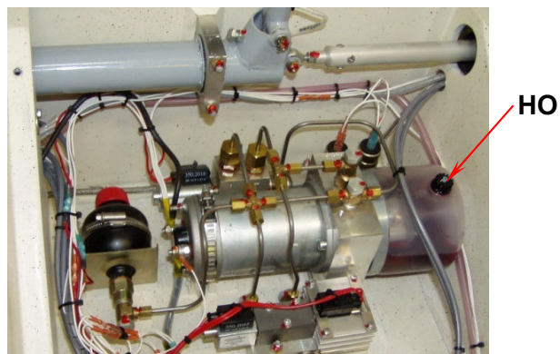
Fig. 2.2.8-3 Operating fluids - hydraulic oil (only model Speed)
