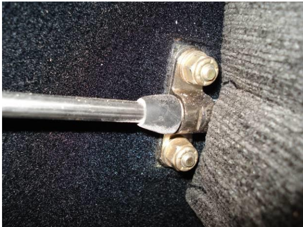
Figure 104 – Trim Cable Clamp Installation (all J-Series)
