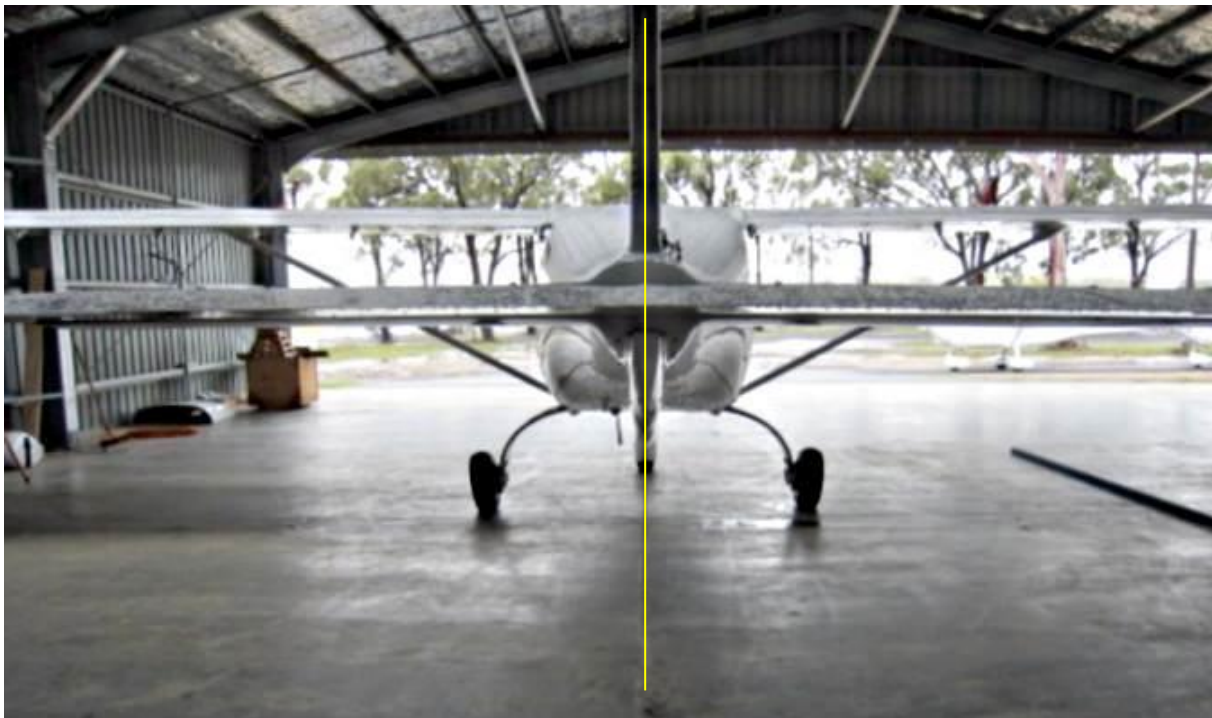
Figure 28 – Wheel Alignment Set Up (all J-Series)
