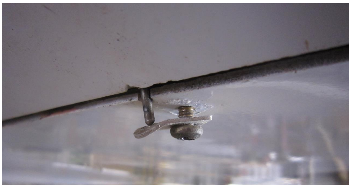
Figure 26 - Hinge pin unlocked
