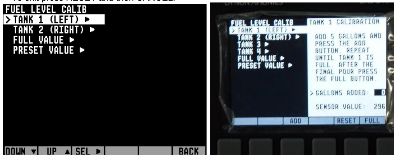
Figure 35 – EMS Fuel Calibration Screens (all J-Series, n/a J120)
