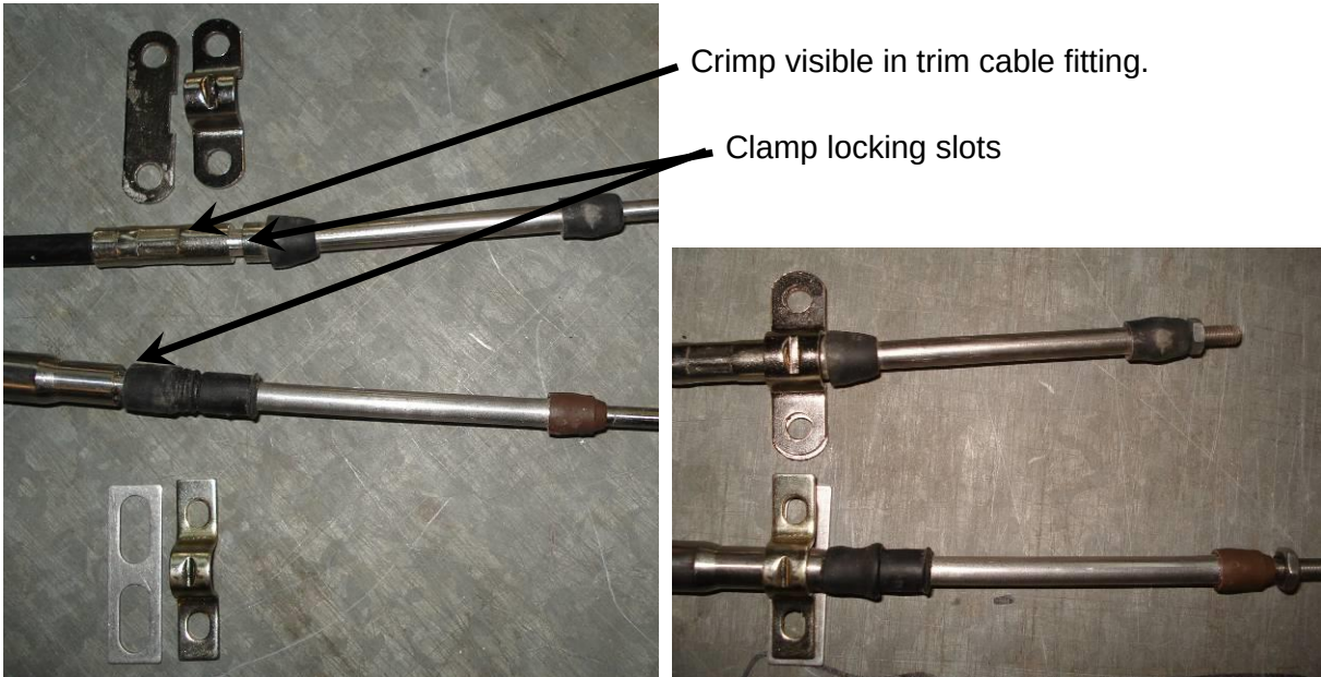
Figure 105 – Cable & Clamp Comparison (all J-Series)
