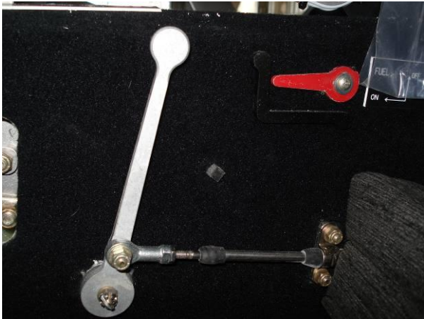
Figure 104 – Trim Cable Clamp Installation (all J-Series)
