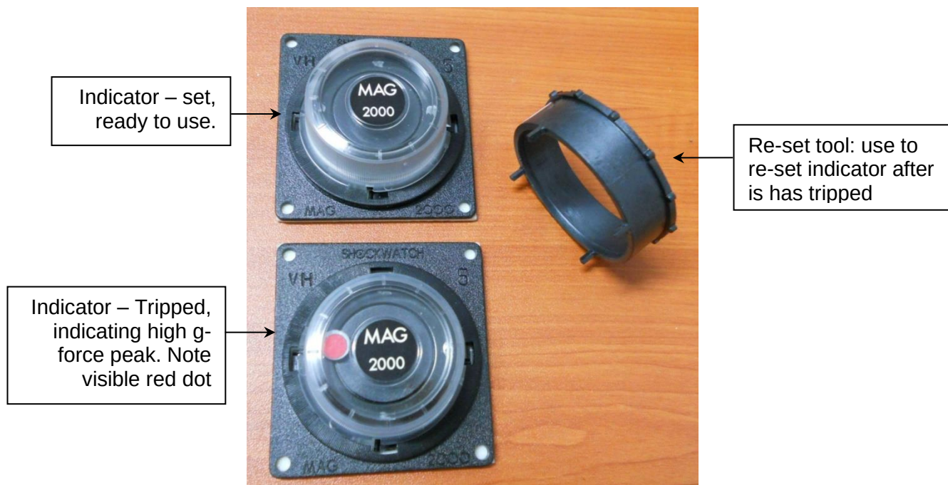
Figure 44 – ShockWatch Indicator (all J-Series)
