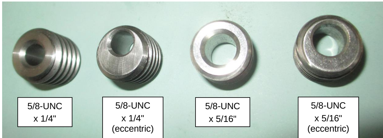
Figure 43 - stainless steel bushes used in Jabiru aircraft wing lugs
