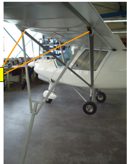
Figure 85: Jacking up the main landing gear with a Kny fork
