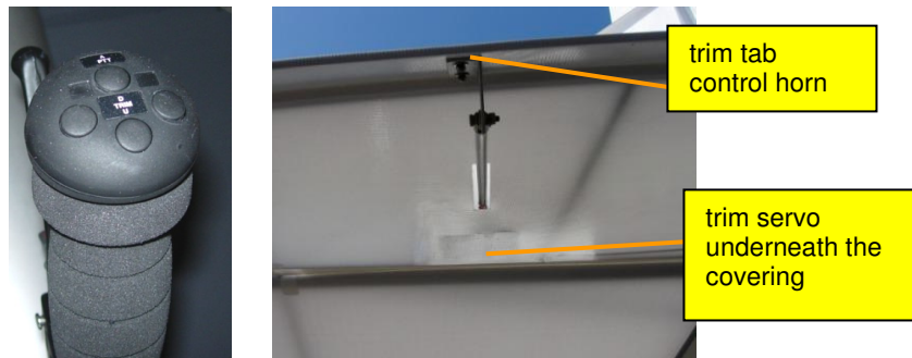
Figure 37: Activation of the electrical trim tab
