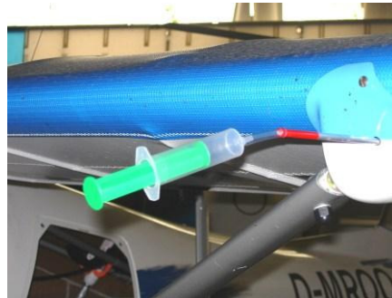
Figure 75: Checking the pitot pressure system
