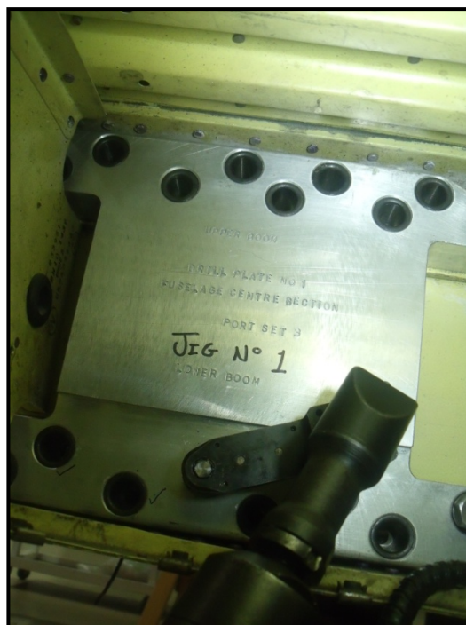
Drill jig fitted inside the stub wing for drilling and reaming operations
