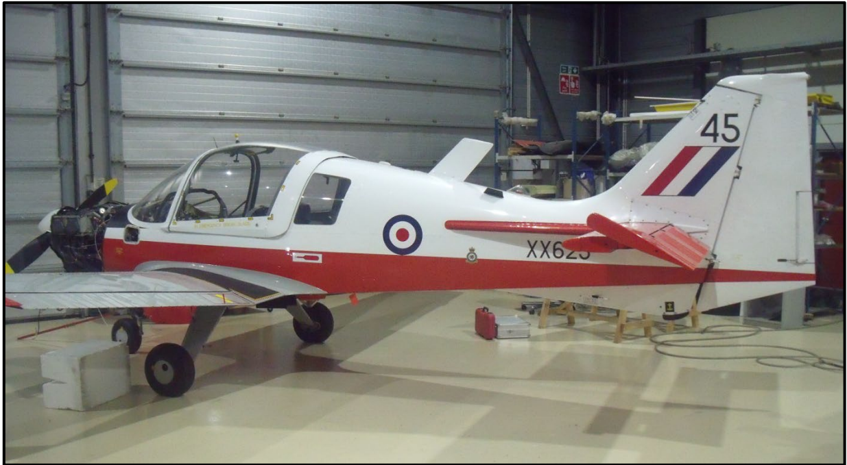
With the wing modification complete, G-UWAS awaits its avionic upgrade. G-UWAS has also assumed the identity XX625 which served with the University of Wales Air Squadron, Royal Air Force St. Athan
