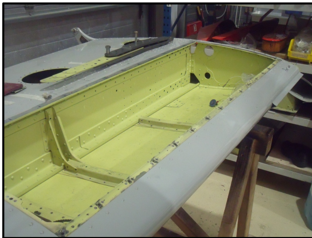
New wing spar straps being drilled and reamed Completed wing tank bay cleaned and primed
