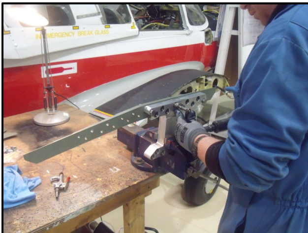
New wing spar straps being drilled and reamed Completed wing tank bay cleaned and primed
