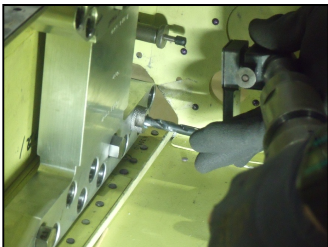
Drill jig fitted to wing spar for drilling and reaming operations
