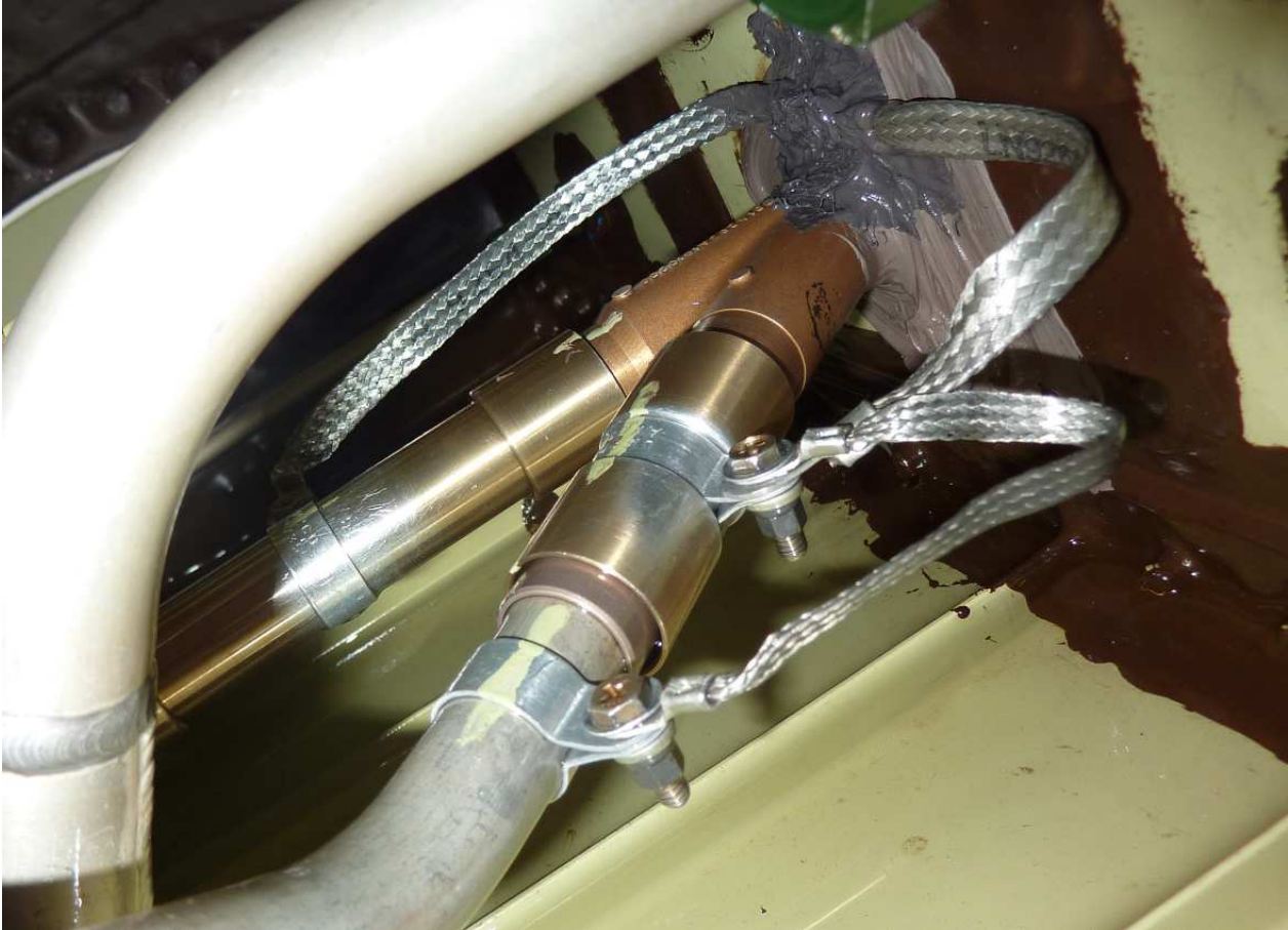
Figure 6: Feeder tank (post-mod)
