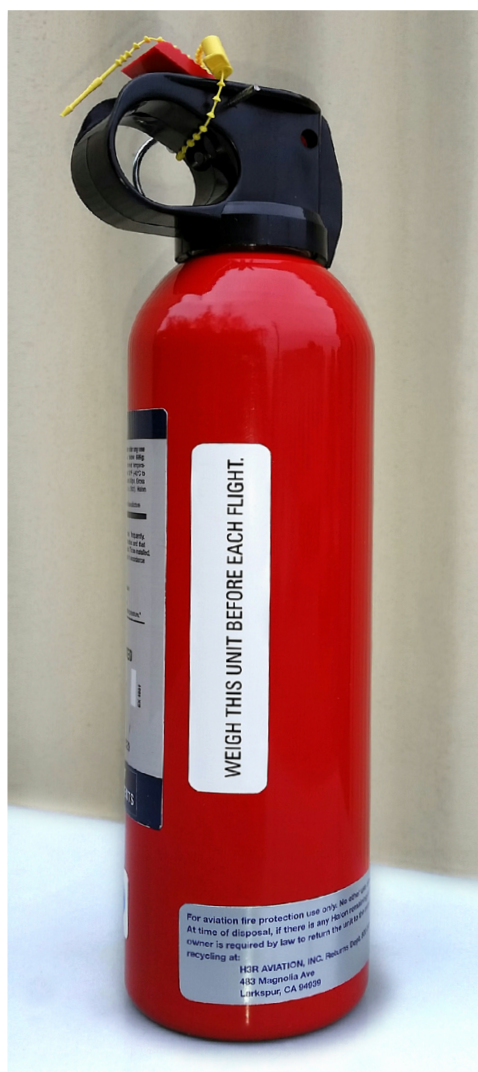
Figure 2 Fire Extinguisher – Piper P/N 459-887 with Label, "Weigh This Unit Before Each Flight"
