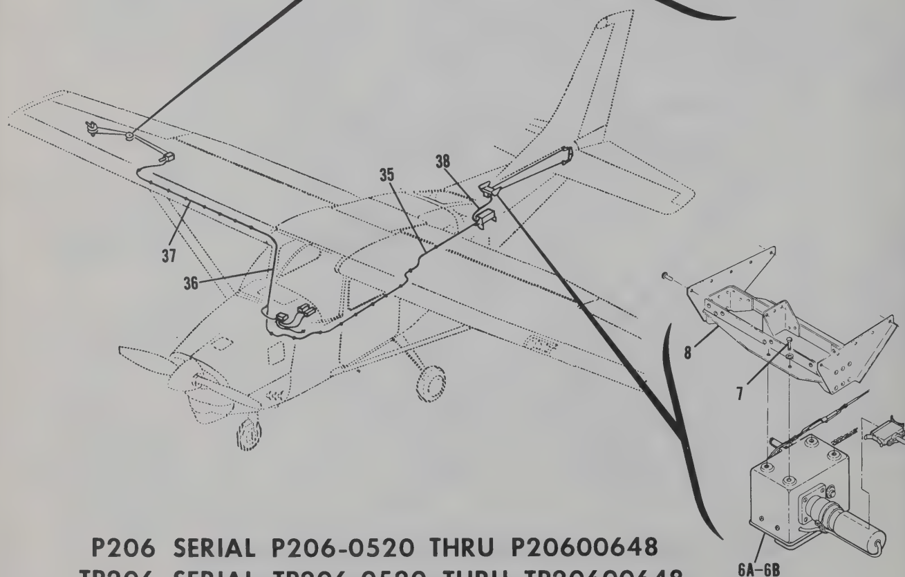
Figure 1-17. Cessna Nav-O-Matic 400 Installation - Model 206 Series Only (Sheet 2 of 2)
