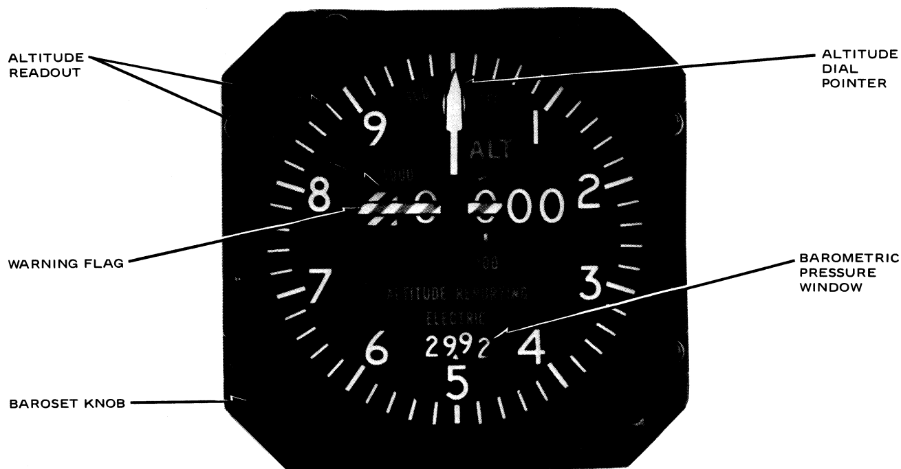
Figure 3-1. Encoding Altimeter, Operating Controls and Indicators
