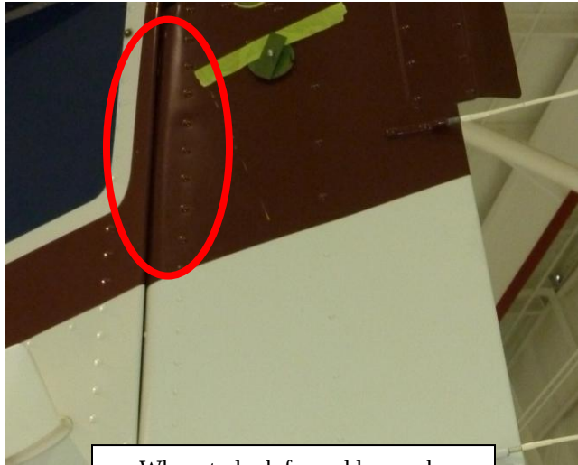
Where to look for rudder cracks
