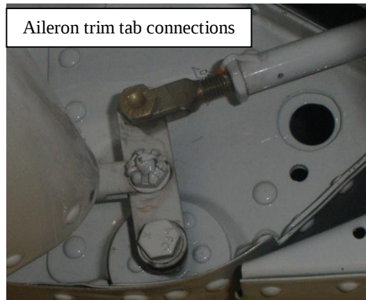
One place to check for interference
