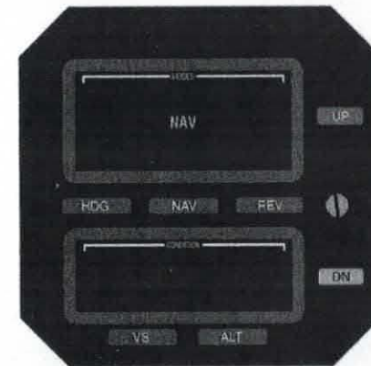
Fig. 3-28. AP Display, NAV Mode Engaged, Before VOR Front Course Intercept
