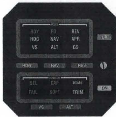
Fig. 2-3. AP Display, All Annunciations Appear
