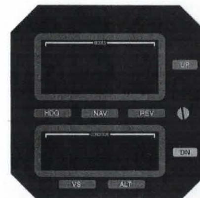
Fig. 2-2. AP Display, Turn Coordinator Failure, RDY Does Not Appear
