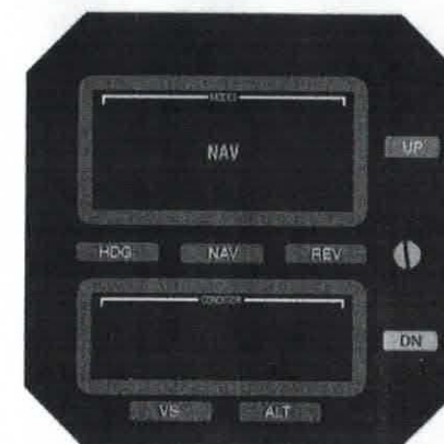
Fig. 3-38. AP Display, NAV Mode Engaged, Before VOR Front Course Intercept
