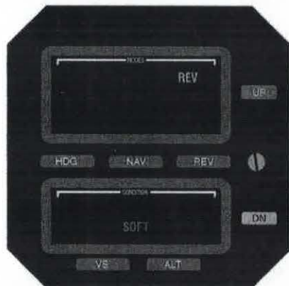
Fig. 3-37. AP Display, REV Mode Engaged, Track VOR Front Course Outbound
