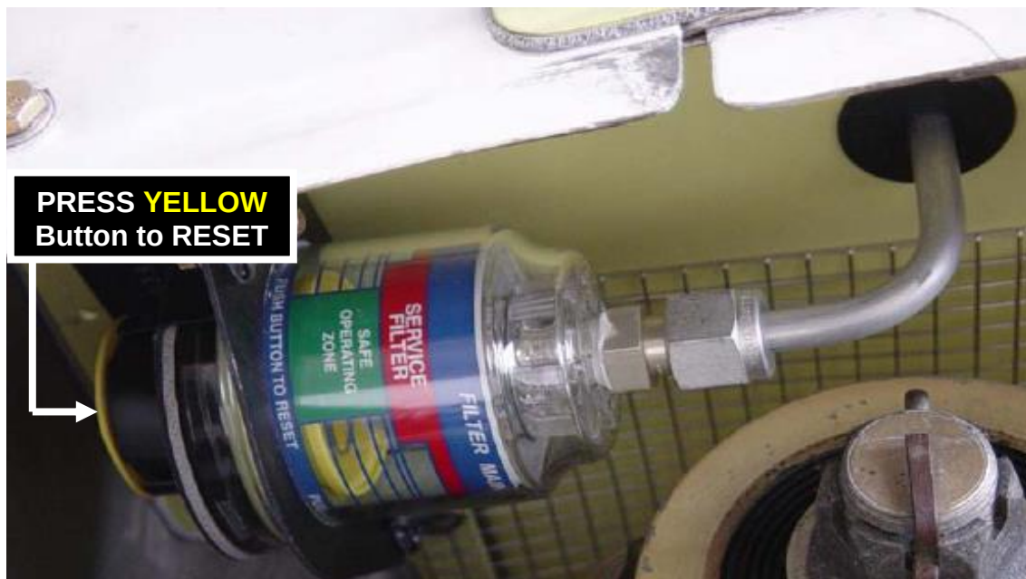
Picture 8-6: FMA / RESET LOCATION - unit is mounted to bottom of IBF floor assembly and is accessed through RH access door on air induction cowl.
