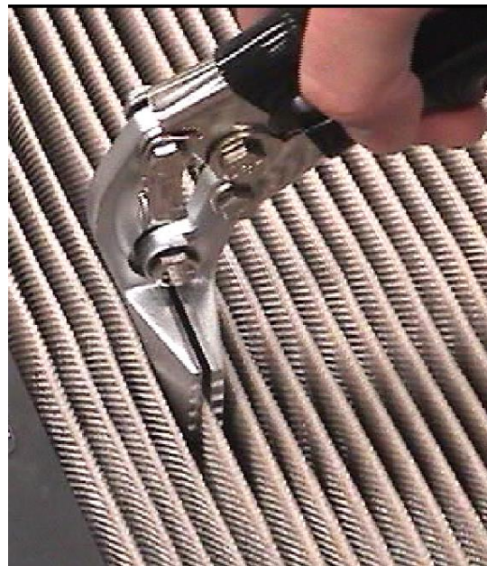
Picture 8-3. HAND SEAMER USED TO STRAIGHTEN OR CRIMP PLEATS
