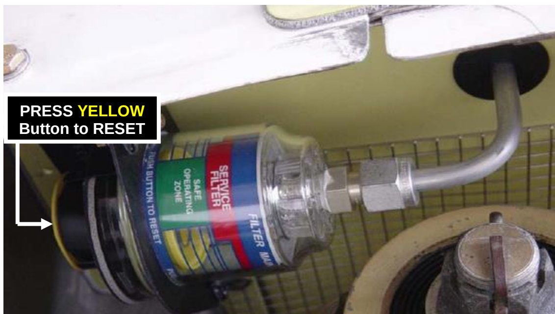
Picture 3-2: FMA RESET LOCATION - unit is mounted to bottom of IBF floor assembly and is accessed through RH access door on air induction cowl.
