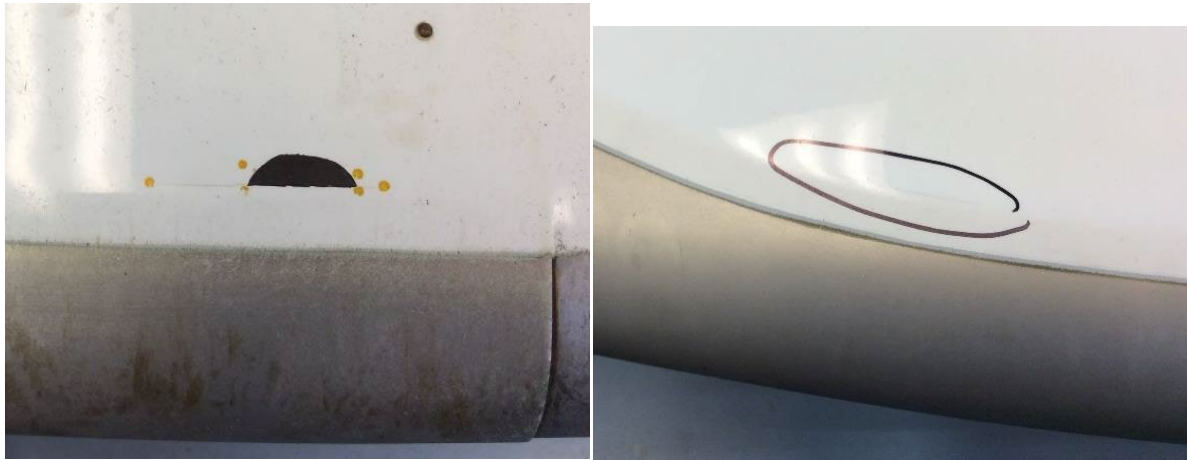
Figure 5-2 Paint Cracks indicating leading edge impact
