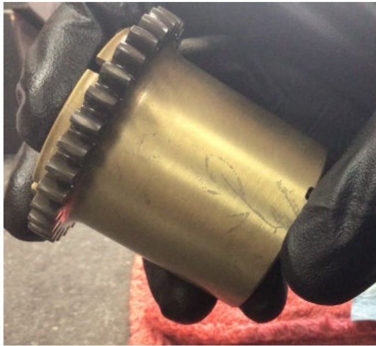
Figure 1 (sheet 1 of 2) - Examples of corrosion on the coupling OD.
