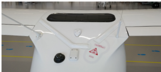
BPRS installation: hatch and belt positioning
