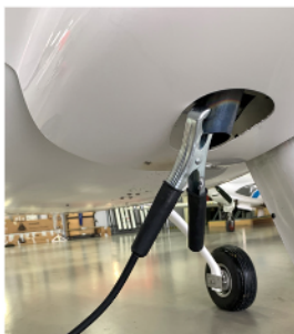
Ground wire connected to exhaust.
