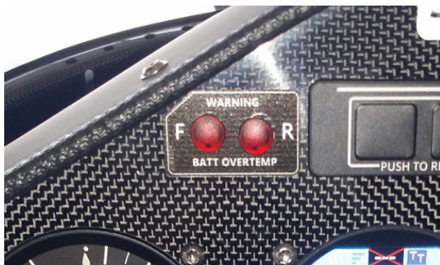
Battery overtemperature warning lights
