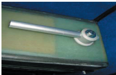
Spar pin - installed
