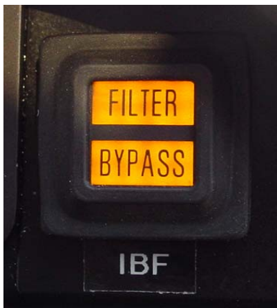
Picture 2: Cockpit Switch/Indicator
