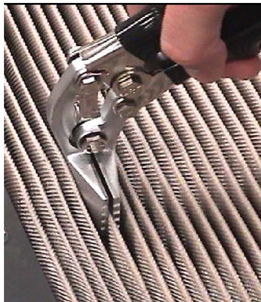
Picture 5: Hand Seamer Used to Straighten or Crimp Pleats
