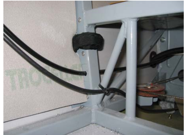
Attacco anteriore Front bridle fitting
