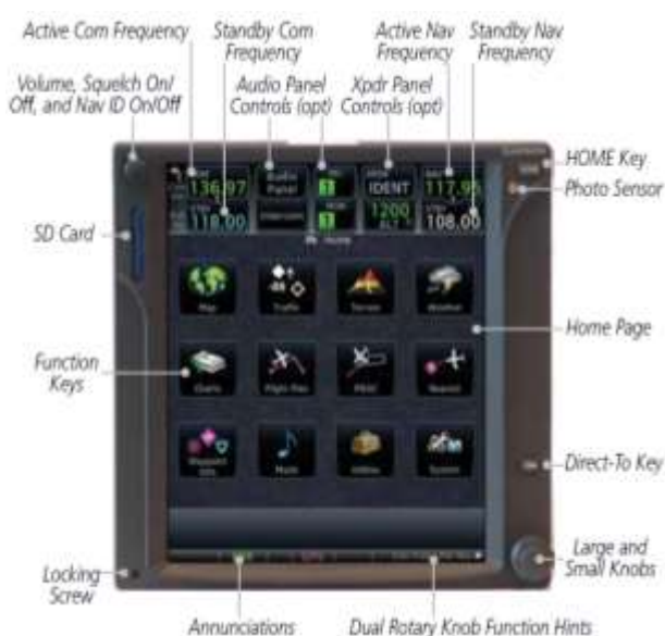
Figure 1- GTN 750 Control and Display Layout
