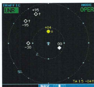
Figure S01-2 - Example of Traffic displayed on MFD
