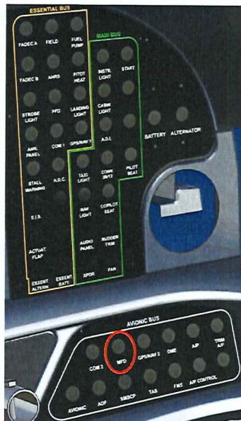
Figure S08 – 3: Breaker Panel
