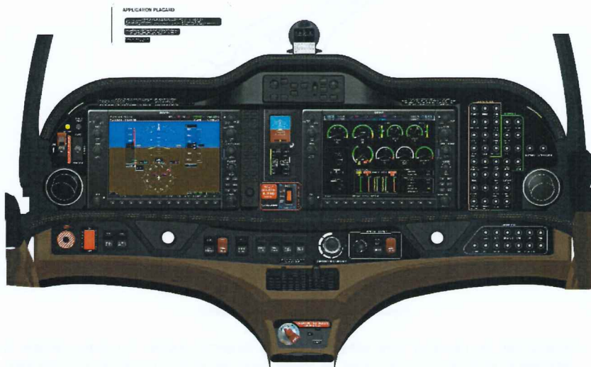
Figure S08 – 8: Cockpit layout with GMC707 unit installed
