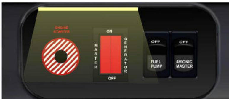
Figure 7-15 - Electrical Main Switches
