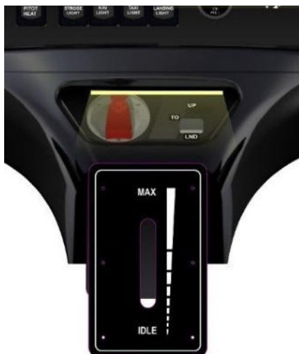
Figure 7-13 - Fuel selector valve control location
