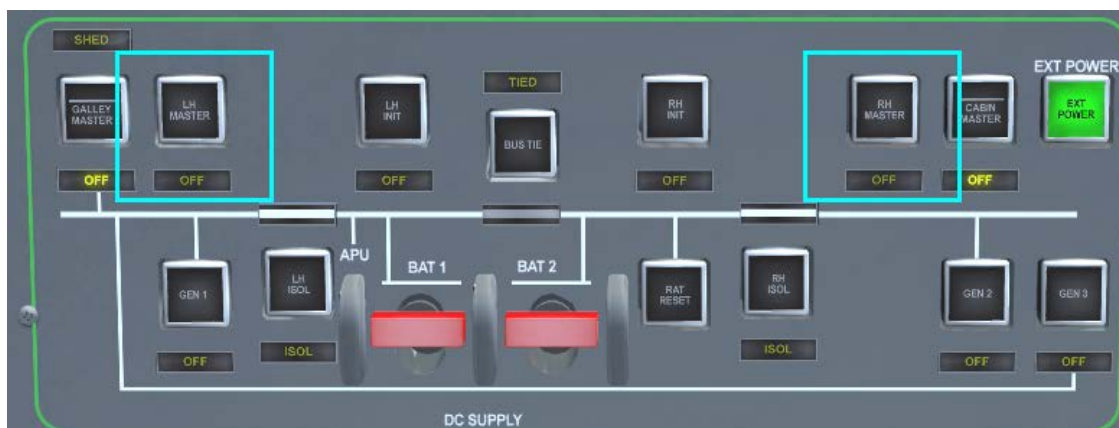
Figure 3 POWER PANEL MASTER BUS CIRCUITS
