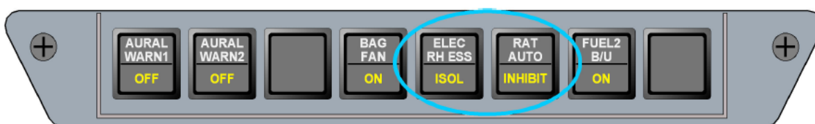
Figure 4 EMERGENCY CONTROL PANEL, ON PEDESTAL
