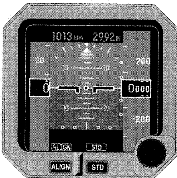
INTEGRATED STANDBY INDICATOR SYSTEM Figure 5-9B
