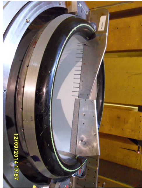
(a) Rotating rake installed over a fan model in the 9x15 LSWT. (b) Close view of dual rotating microphone rakes.
