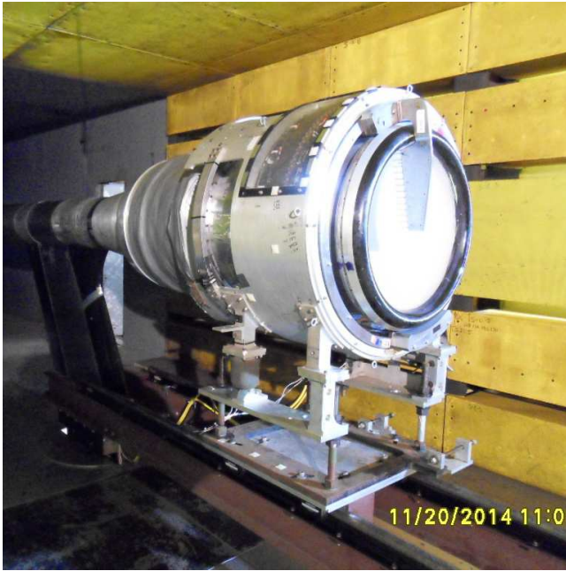
(a) Rotating rake installed over a fan model in the 9x15 LSWT. (b) Close view of dual rotating microphone rakes.
