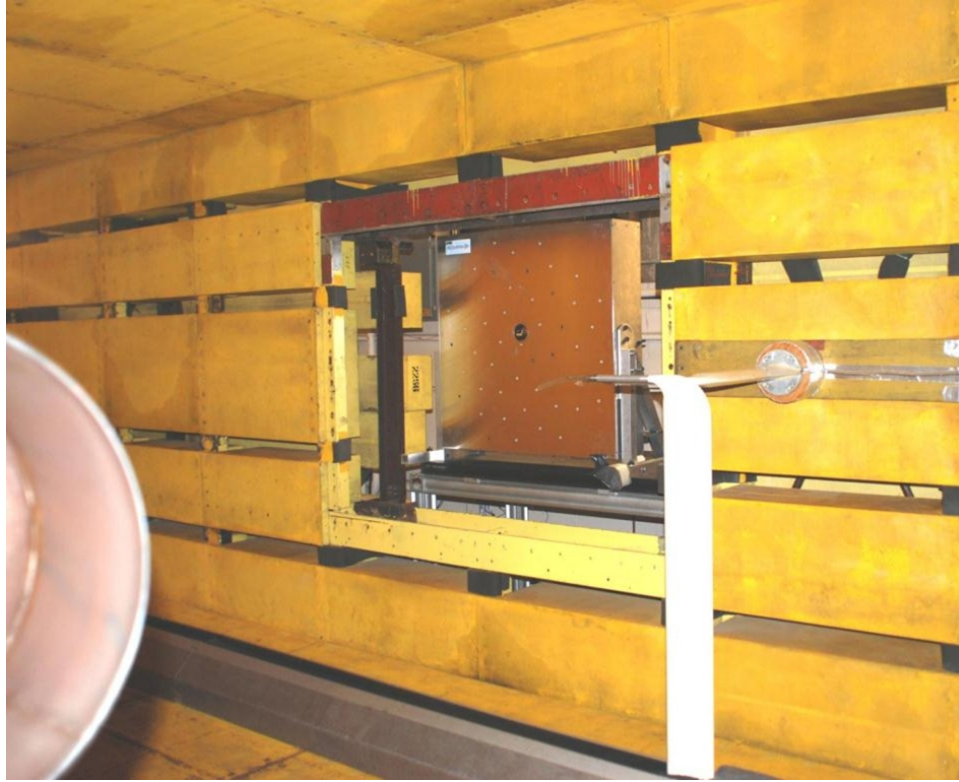
Figure 15: Optinav Array-48 installed in the 9x15 LSWT.
