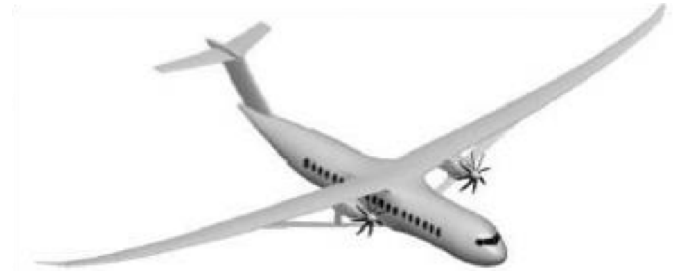
NASA AATT PT - Unducted Propulsor Research (open-rotor engine architecture)
