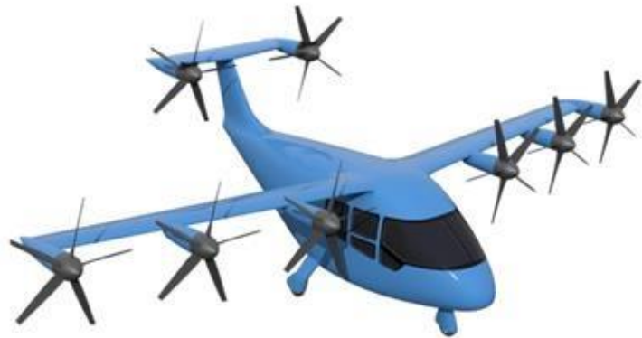
NASA UAM - Tiltwing Concept Vehicle (cruise configuration)
