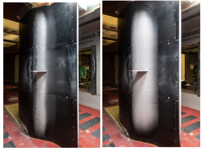
Figure 19. Images showing extent of ice on the suction side of the test article where tests were conducted at 4^\circ AoA, and MVD varied from 18 \mu\text{m} (left) to 90 \mu\text{m} (right). From Block B in Table 2, Test Run IDs UG3541 and UG3542 respectively.
