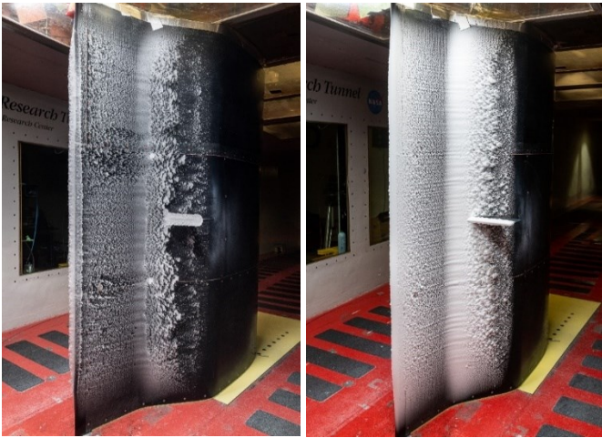
Figure 21. Images of ice accretions from the air temperature sweep with a glaze ice accretion on the left ( T_0 = -3\text{ }^{\circ}\text{C} ), and rime ice accretion on the right ( T_0 = -17\text{ }^{\circ}\text{C} ). From Block D in Table 2, Test Run IDs UG3531 and UG3534 respectively.
