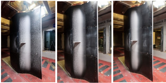
Figure 17. Images showing extent of ice on the suction side of the test article where AoA varied from 0^\circ (left), 2^\circ (middle), and 4^\circ (right). From Block E in Table 2, Test Run IDs UG3538, UG3539, and UG3540 respectively.
