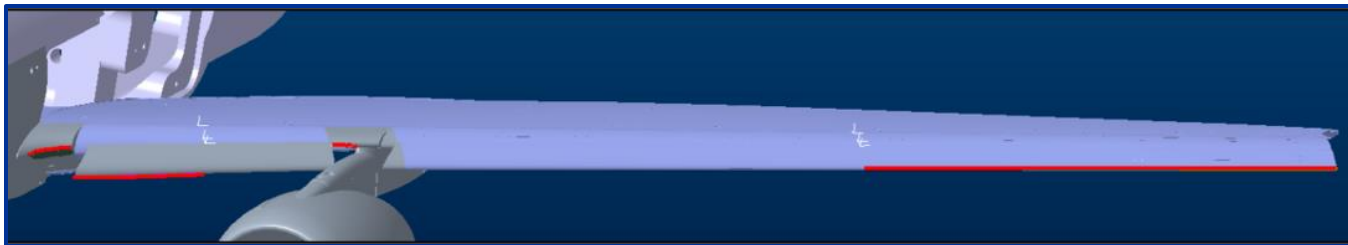
Schematic of the artificial ice shapes (Red) on the High Lift Common Research Model
