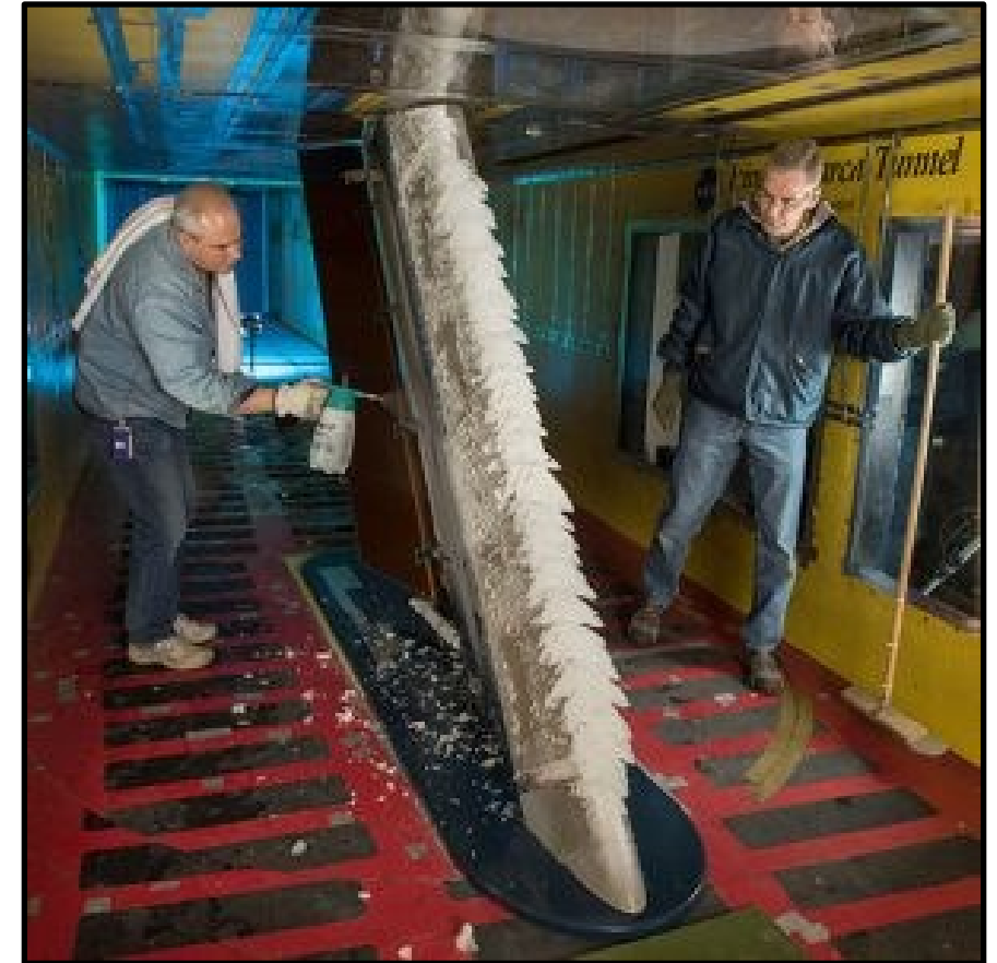
IRT Test Section
