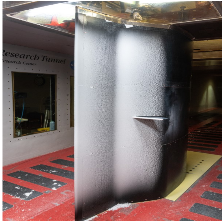
Supercooled liquid ice accretion on SIDRM
