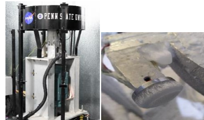
Centrifuge shear test and ice coupon on centrifuge arm
