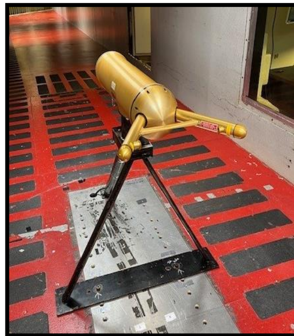
OAP-230Y: 50 to 1500 \mu\text{m} OAP-1D2DY: 50 to 3200 \mu\text{m}
