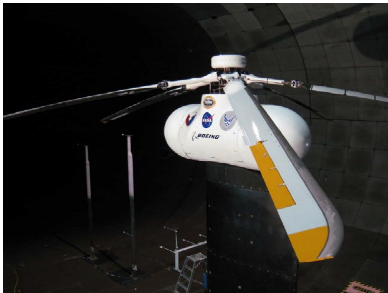
Figure 1f: Close-up view of the SMART rotor, blade, and flap in the tunnel.
