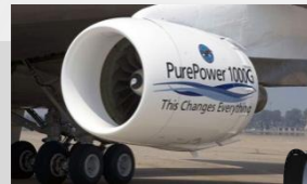
P&W PurePower 1000G Geared Turbofan
