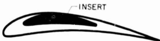
(C) VANE 3. INTERNAL INSULATING INSERT
